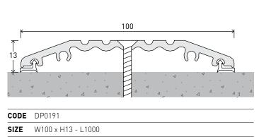
FIXING Screw-fixed (screws supplied)
